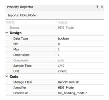
Based on these settings, the code generator imports the declaration for external variable HDG Mode from header file roll heading mode.h.
